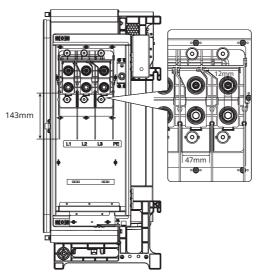
Prepare the copper to aluminum wiring terminal reffering to the dimension requirements above. Contact the after-sales service for the copper to aluminum wiring terminal for AC cable with a cross sectional area of 400mm<sup>2</sup>.
