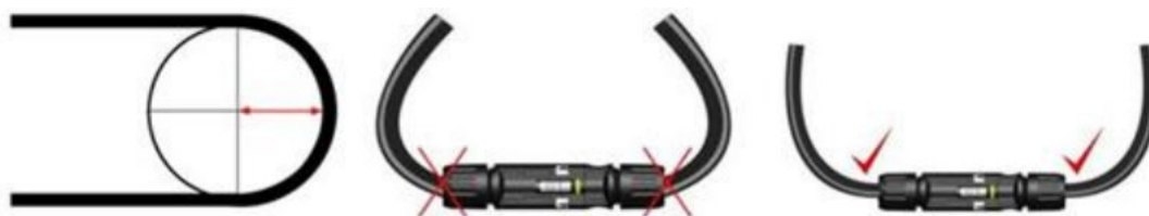
FIGURE 31 MINIMUM BENDING RADIUS OF THE CABLE
