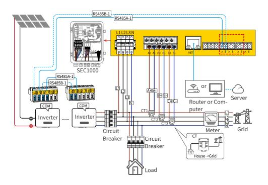
Based on the external CT test current, the recommended CT specification are:
