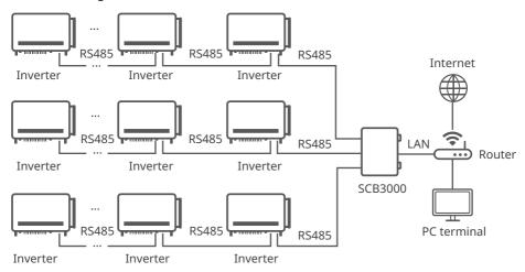
Connect the RS485 port of the inverter to the Data Logger. The total length of the connection cable is less than 1000m.
