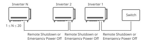
Connecting the Remote Shutdown and Emergency Power Off Communication Cable
